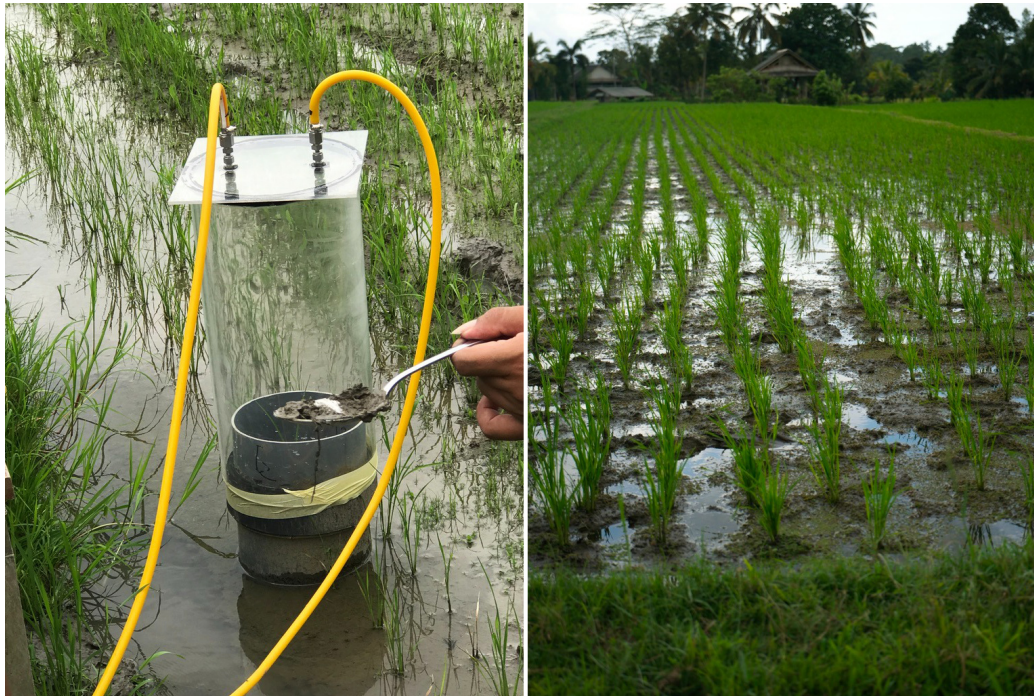
A (Left) Picarro gas analyzer used to measure the emission of greenhouse gases in a paddy field. (Right) A drained rice paddy field. Images by Steve Lansing
